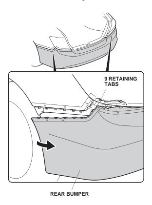
With the help of an assistant, remove the rear bumper. Set the rear bumper on a blanket to prevent damage.
