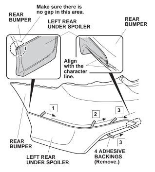
12. Remove the four adhesive backings in the order shown. Press the left rear under spoiler firmly against the rear bumper with the palms of your hands to set the adhesive. Tighten the two female clips loosely installed in step
