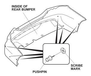
3. While wearing eye protection, drill the two lower pierced marks with a 3 mm drill bit, then enlarge the holes with a 10 mm drill bit.
